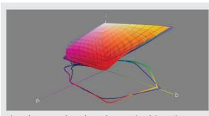
The color gamut chart above shows in detail the wider gamut of reds that the HP Designjet Z3200 Photo Printer (in solid) achieves in comparison to one of its competitors. HP Premium Instant-dry Gloss Photo Paper was used for the demonstration.
