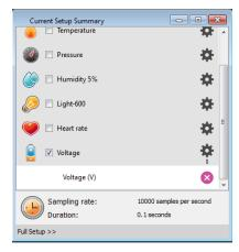
5. Click Full Setup, located at the bottom of the Current Setup Summary window to program the data logger's sample rate, number of samples, units of measurement, and other options
