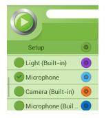
5. Check the icon next to the sensor (  $\circledast$  ) to enable it for logging
